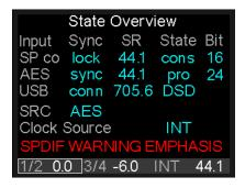
The status bar always shows the current volume setting of outputs 1/2 and 3/4, the currently selected output for the Volume knob by a marker around the outputs, the current clock source, and the current sample rate. In case of Sync problems the sample rate will either fluctuate or be shown in red – or both. This information is available in nearly all screens, and helps to get a quick overview of the current state. The State Overview screen now extends this information in great detail.
