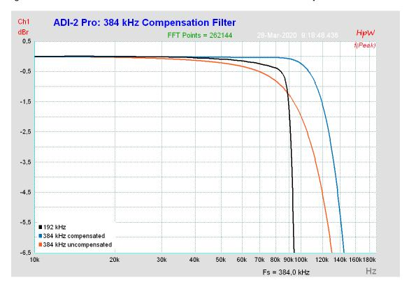
The blue curve shows the effect of RME's digital compensation filter at 384 kHz sample rate. The frequency response is now near flat up to 90 kHz, with minimal decrease in the area of the 192 kHz sample. With this filter the ADI-2 Pro can easily measure any 192 kHz (and lower, of course) operated device with high accuracy, at fractions of a dB.
