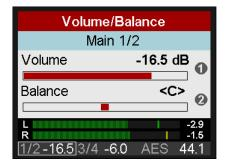
The status bar at the bottom of the display shows the current dB value of both volume settings. A white rectangle around it (marker) indicates which volume the big encoder is currently set to control.
