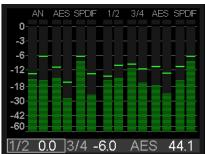
All level meters (vertical and horizontal) of the ADI-2 Pro are peak level meters with peak hold function, band limited to 40 kHz even at higher sample rates. OVR (Over) are displayed in red color at the upper end. For digital I/Os, Over appears when the signal is at the maximum possible level. As usual in digital audio, Over is already displayed even if there is no real overload.
