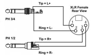
The use of a 4-pin XLR male connector on the phones side is quite popular. The diagram to the right shows how an adapter cable can be used to connect the ADI-2 Pro phones outputs, using two stereo TRS plugs and one female XLR connector.
