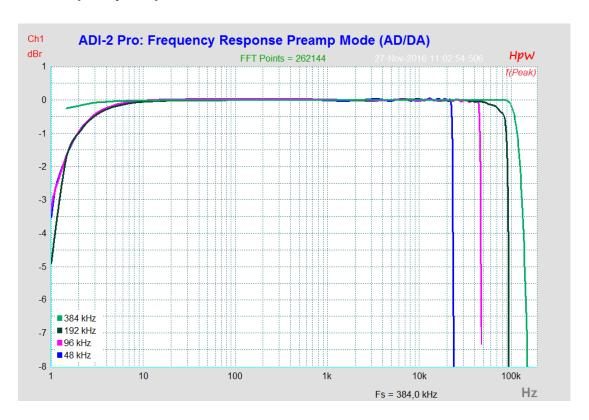
Note: 44.1 kHz to 192 kHz measured with filter Sharp on AD and DA..
