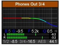
As the measurement below shows these settings compensate the DAC's de-emphasis with 0.1 dB accuracy.
