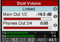
In the Dual Volume screen, both outputs can be muted by pushing encoder 1 (B) and encoder 2 (T) respectively.
