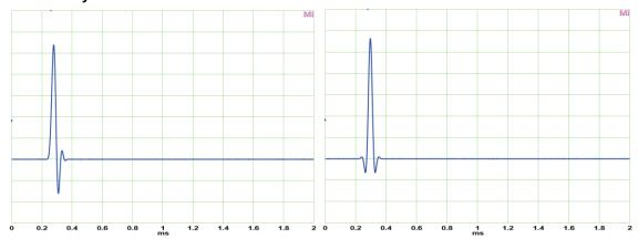
The screenshots above show the analog output signal of the DAC filters, stimulated by a digital single sample impulse at 44.1 kHz sample rate. While Slow has the most perfect response, it looses around 1.2 dB already at 15 kHz, see chapter 34.14. Both Short Delay are IIR filters, the other two are FIR type. FIR is phase linear over the whole frequency range.
