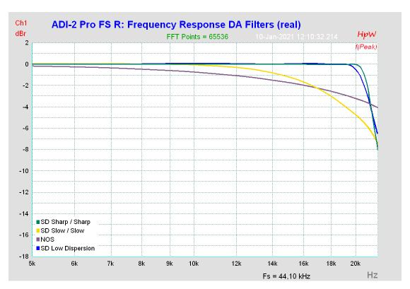
Note: Sharp/SD Sharp and Slow/SD Slow are congruent. NOS shows a very early drop. SD Low Dispersion is almost as linear as Sharp/SD Sharp.
