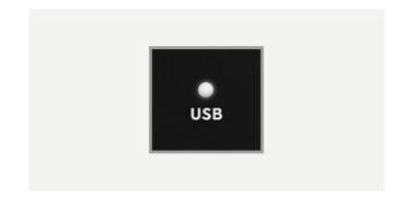
The white USB LED indicates connection via USB to your device. A solidly lit light means that there is stable communication between iD4 and the device.
