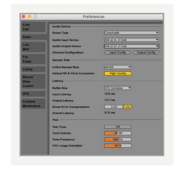
If you are monitoring your inputs using the Monitor Mix knob, then you can keep the buffer size reasonably high to reduce the strain on your computer. In this case, you also need to make sure that input monitoring is turned off on the track in Ableton.
