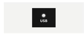
If at any time the USB LED turns off during normal operation please check all connections and if further problems develop, please contact **Audient Support.**
