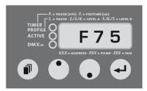
Fig. 10: Adjusting the output value for the fan.
