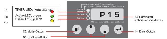
Fig. 6: Adjusting the performance of the fog generator
