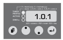
Fig. 19: Adjusting the Pre-Runtime
