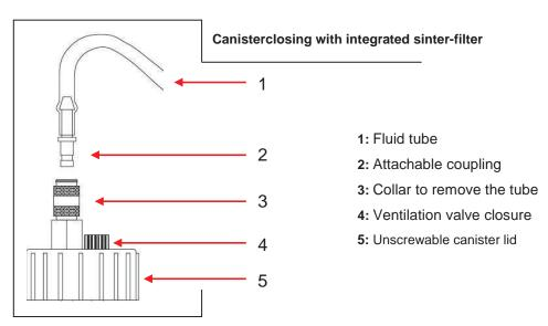
Fig. 4: Canisterclosing with integrated sinter-filter
