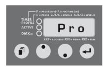
Fig.: 12: Switching to Profile mode
