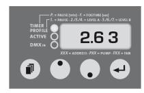
Fig. 20: Adjusting the pump value.
