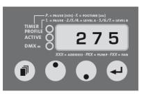
Fig. 11: Adjusting the DMX start address.
