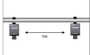
Take the width of your cloth or object that has to be dropped and determine where the first and last Power Drop have to be suspended.
