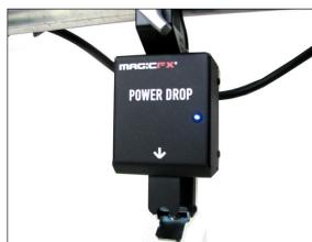
Connect the Power Drops to a 230v electricity source to check if all Power Drops have been connected properly. When everything is connected properly the blue LED indicators will light up on the Power Drops.
