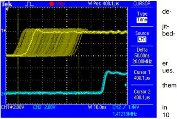
Common interface jitter values real world applications are below ns, a very good value is less than 2 ns.
