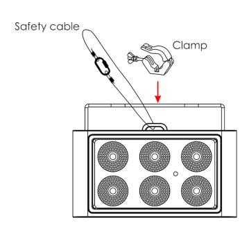
The Cameleon Flood 6NW can be placed on a flat stage floor or mounted to any kind of truss with a clamp.
