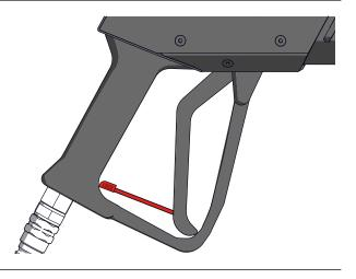
**5** Disconnect the CO2 hose from the CO2 quick connector on the pistol.
