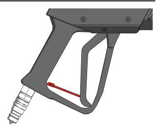
2 Connect the CO<sub>2</sub> hose to the CO<sub>2</sub> quick connector.
