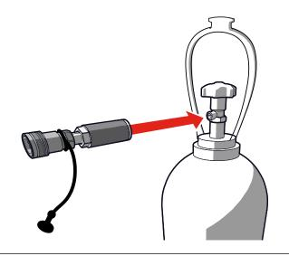
4 Connect the  $CO_2$  hose to the  $CO_2$  bottleto-hose connector on the  $CO_2$  cylinder.
