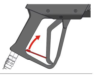
**3** Squeeze the handle to release the remaining pressure.
