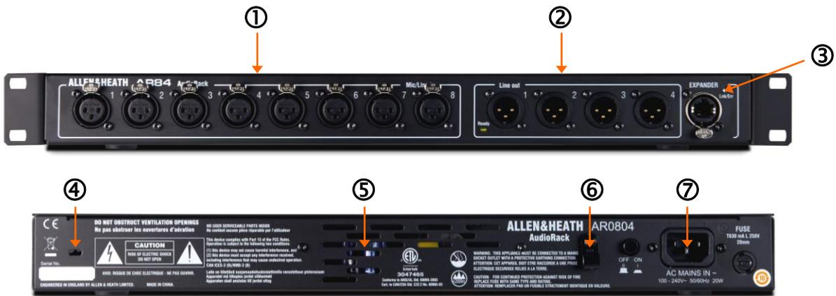
① **Input sockets** 8 balanced XLR inputs for microphone and line level sources. The preamps are built into the AR84 rack and their Gain, Pad and 48V phantom power is remote controlled from the mixer via the digital link. The outputs of the analogue preamps are converted to digital format and transported via a Cat5 cable to be processed and mixed at the mixer.
