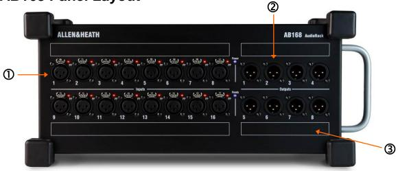
**U** Input sockets 16 balanced XLR mic/line inputs with +48V Phantom Power indicator. The preamps are built into the AB168 and their Gain, Pad and 48V phantom power are remote controlled from the mixer via the dSNAKE link. The outputs of the analogue preamps are converted to digital format and transported via dSNAKE to be processed and mixed at the GLD, SQ or Qu mixer.
